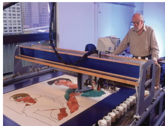
Fig 1. AARON: a robot used by artist Harold Cohen to make abstract images autonomously using a routine programmed to mimic Cohen’s own style. Source: technologyreview.com .
